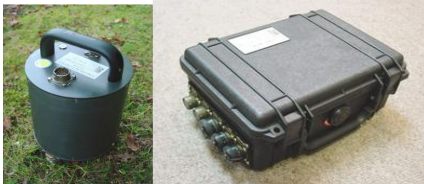
Figure 1. - Broadband three-component CMG-6TD seismometer and EAM recorder
